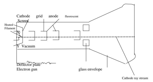
The cathode rays oscillope is used for studying all types of wave forms especially the alternating current wave forms and to measure frequencies and amplitude of voltage of electronic devices.
