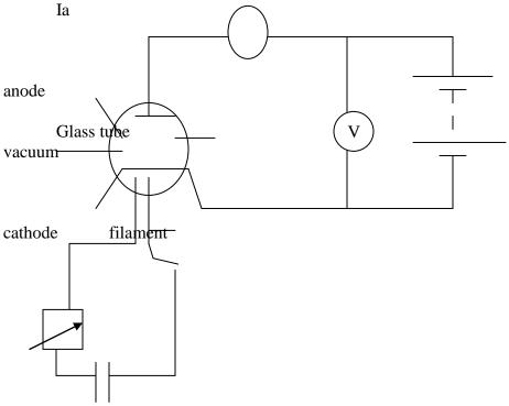
The filament supplies free electrons when heated by the current from the battery (E), when the anode is made positive in potential with respect to the cathode, electrons low towards the anode and constitute the anode current (Ia) which is registered by the milliameter.
